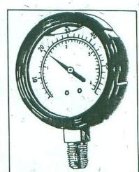
An accurate pressure gauge is one of most important tools that you need to manage a micro-irrigation system.
