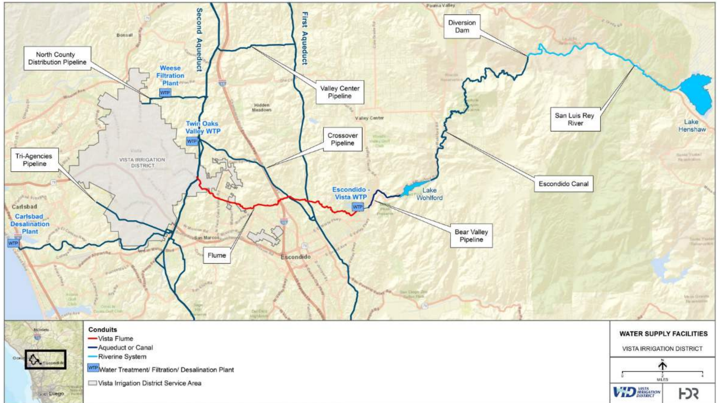
Figure 1-2. Regional water supply facilities; 2016 VID master plan
