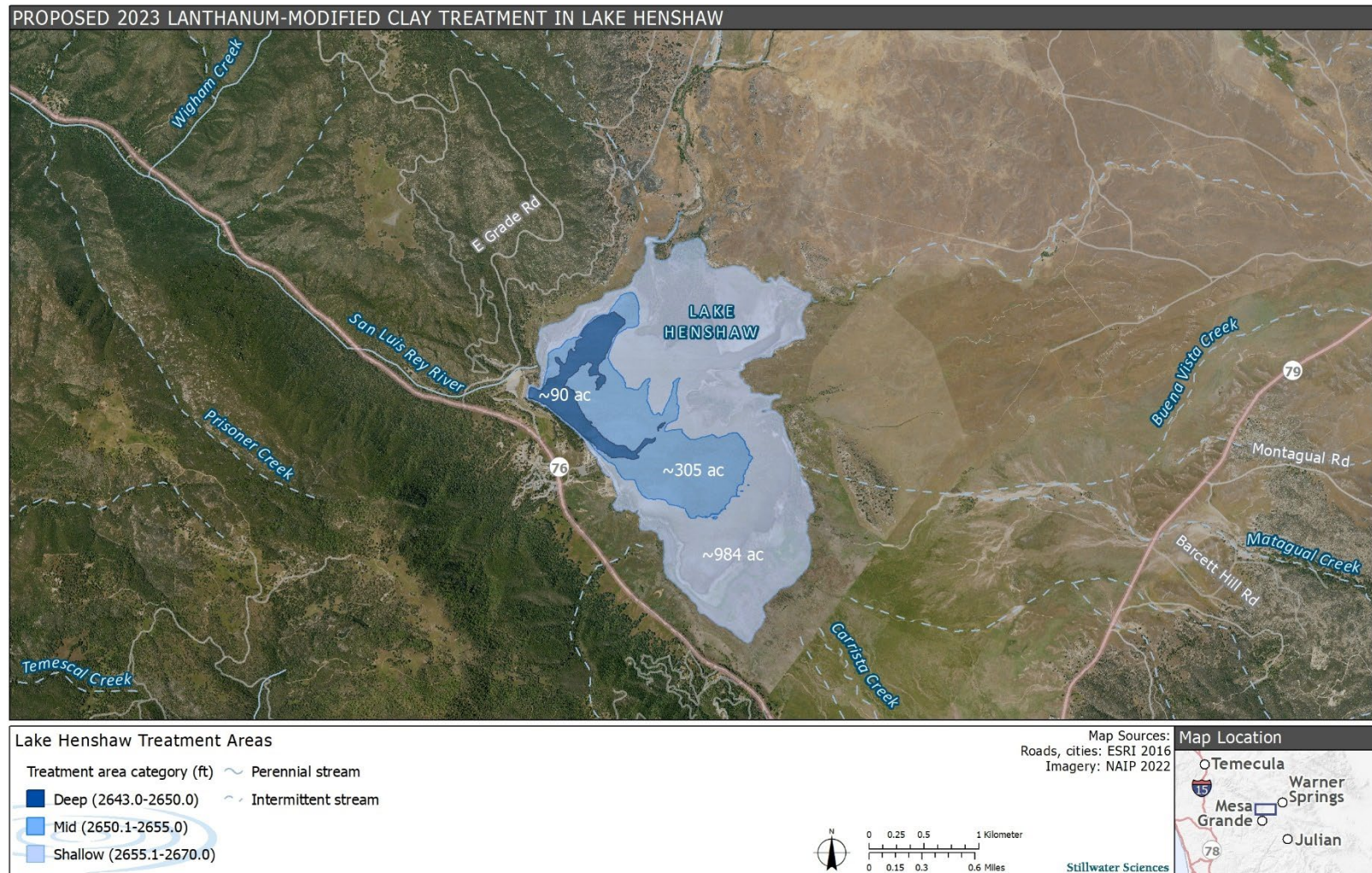
Figure 3-1. Lake Henshaw treatment areas according to overlying water depth sediment categories, deep (dark blue), mid (blue), and shallow (light blue). Acres reported here are estimated based on lake bathymetry (2018) and assume lake elevation at 2,670 ft, storage at 14,580 ac-ft.
